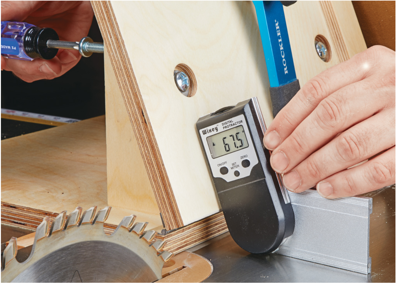
Lock it Down. First, verifying the angle of the platen with a digital angle guide.
